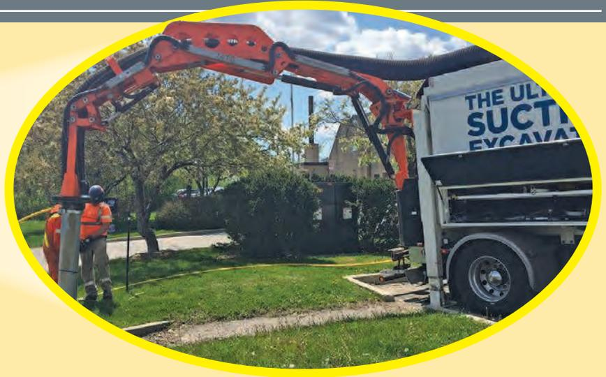
“Productivity levels for the MTS dry suction equipment rivals that of a typical hydrovac in most instances and all without generating any wet spoils,” Donoahue says.
